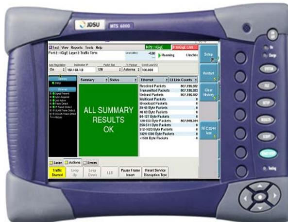
**Figure 13** T-BERD/MTS 6000AV2 with MSAM user interface
