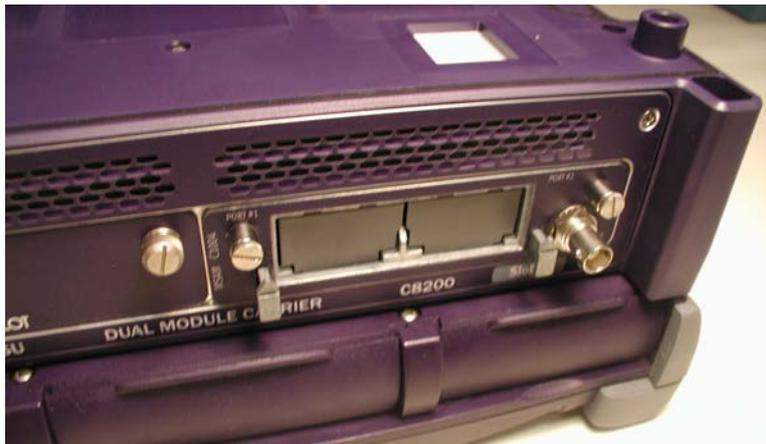
**Figure 29** DMC with CSAM inserted (left) and MSAM v2 inserted (right)
